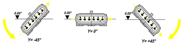
SINGLE AXIS TILT SENSOR ( $\pm 180^\circ$ ) - Z AXIS
